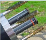
The TurbiTechw $^2$  LS Sensor is designed to monitor the levels of Suspended Solids or Turbidity typically found in Final Effluent from municipal and industrial wastewater treatment plants. It is also capable of monitoring solids in the intake to both effluent and drinking water treatment processes. The normal operating range is between 0 - 50 and 0 - 500 FTU, a version of the sensor is available that extends the range to 0-1,000 FTU.
