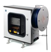
The ASLD 2200 is a fully automatic sludge blanket level detector primarily designed for the water and waste water industry but could be applied to other types of process. It utilises a servo-driven sensor which continually tracks the settled interface and produces a 4-20 mA output which is proportional to the depth of the blanket.
