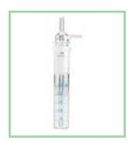
Impingers are special glass tubes designed to collect airborne contaminants by bubbling the sampled air at a high flow rate through a method specific absorbing liquid inside. The liquid used can then be analyzed to determine airborne contaminate levels.
