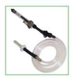
For gas and vapour sampling, a volume of air is adsorbed onto a sampling medium held in glass sampling tubes. To enable a high flow sampling pump to operate at low flow rates required (2-200ml/min) a low flow adaptor assembly is used which acts as a throttle to slow the sampling rate down on a standard air sampling pump. (For range of tubes refer to separate section of the catalogue.)
