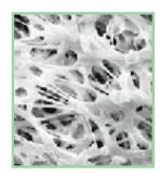
Top quality filter for measuring dust, silica and chromium. There is a low tare weight so a lower sample weight is required and they have a low moisture absorption.
