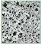
Suitable for further analysis other than gravimetric. Primarily used for air sampling of metals and fibres (e.g. Asbestos). MCE is stronger than GFA so ideal when further post analysis is required other than weighing.
