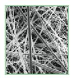
Often referred to as depth filters, these ideal for general gravimetric air sampling and analysis. Available unweighed or pre-weighed. Use for dusts when no further analysis other than weighing is required.
