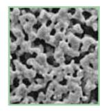
Made from almost pure silver these filters can be cleaned and reused for economical air sampling.
