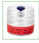
Each cassette contains 2 filters which are matched in weight. After sampling, the user will weigh both filters. The difference in weight of the two filters will determine the sample amount.
