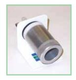
Sampling for asbestos involves specifically designed sampling heads and cowls together with special gridded filters which are later inspected visually or via Scanning Electron Microscope.
