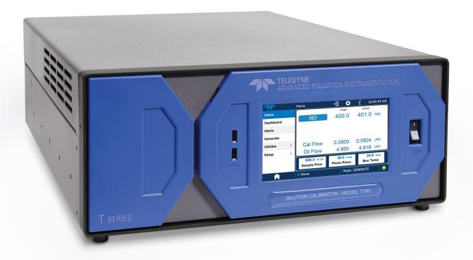
The Model T700 uses highly accurate mass flow controllers for a wide range of gas delivery concentrations and may be equipped with an optional UV ozone generator, photometer, and gas phase titration (GPT) chamber for accurate, dependable ozone calibrations.
