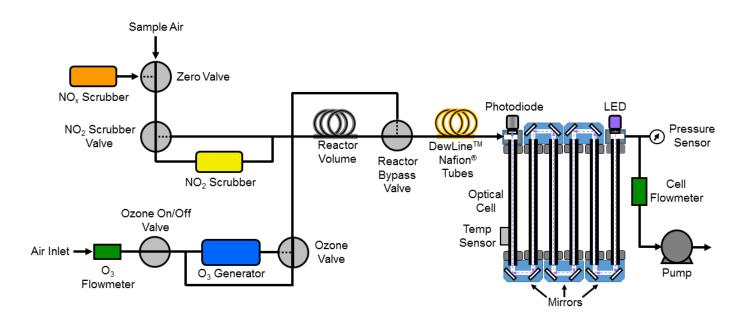
Fig. 1. Simplified schematic diagram of the Model 405 nm NO<sub>2</sub>/NO/NO<sub>x</sub> Monitor.
